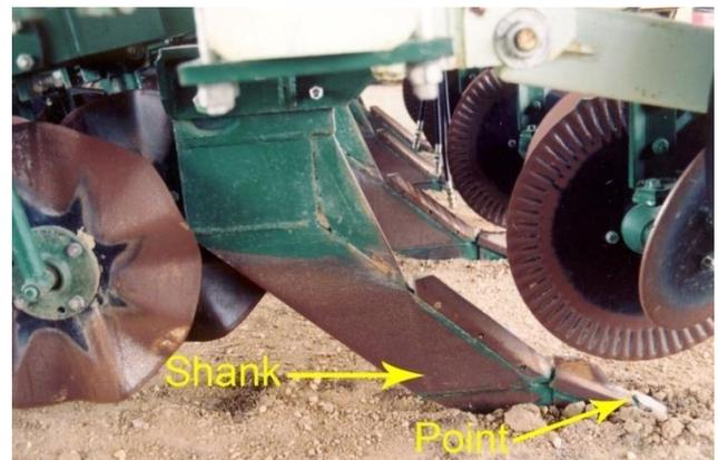
Figure 1. KMC subsoiler shank with principal parts labeled.
