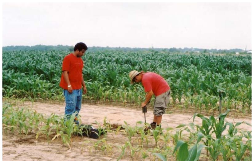
**Figure 5.** Interns learned to measure soil bulk density and interpret the results. Information gained from bulk density provides insight about the physical condition of the soil with respect to the ingress and transfer of air, moisture, and heat.
