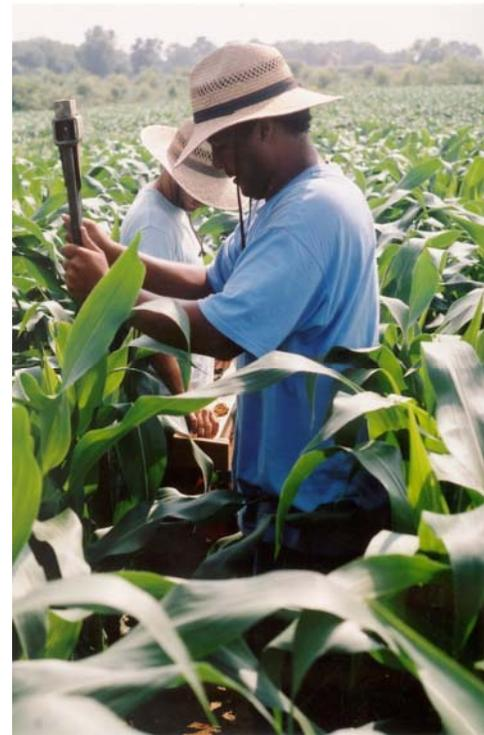
**Figure 3.** Sampling to a depth of 45 cm using a drive hammer and tube. Obtaining a representative sample is an important aspect of diagnostic testing.
