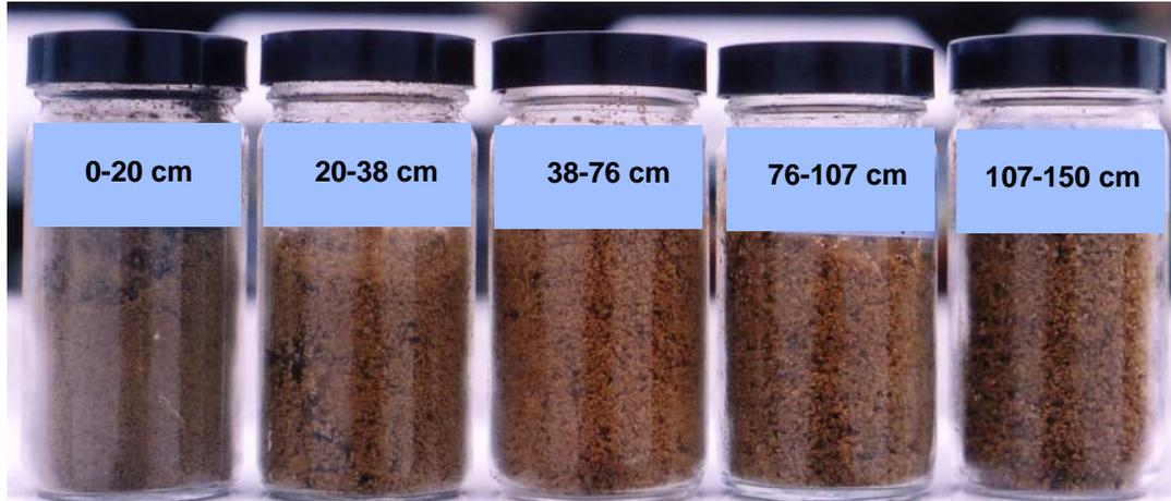
**Figure 8.** Soil samples recovered from the 0-150 cm depth at the problem site. Note the uniformly coarse texture throughout the profile of this Tarboro loamy sand.
