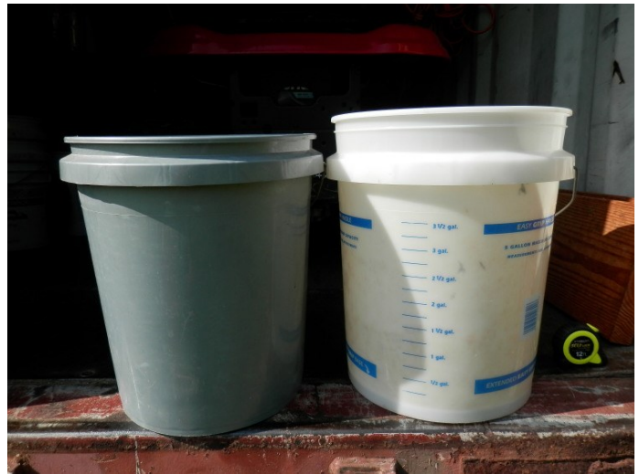
Figure 1. Two “5-gallon” buckets from the same manufacturer but with different brim capacities. Where’s the 5-gallon mark?
